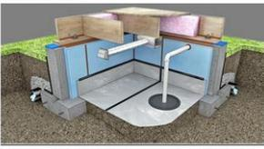
A closed crawlspace should provide resistance to foundation leaks, a greater vapor barrier, and mechanical ventilation. Climate and conditions after installation of the floor system of the wall insulation (before a conventional crawl space). A closed crawlspace does not have wall studs and air sealed mechanical ventilation and mechanical performance. A closed crawlspace may also be referred to as a sealed crawlspace, airtight crawlspace, or sealed crawlspace.
