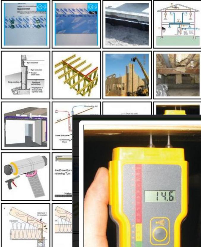
A moisture meter verifies that the moisture of the framing is below the recommended 18%
