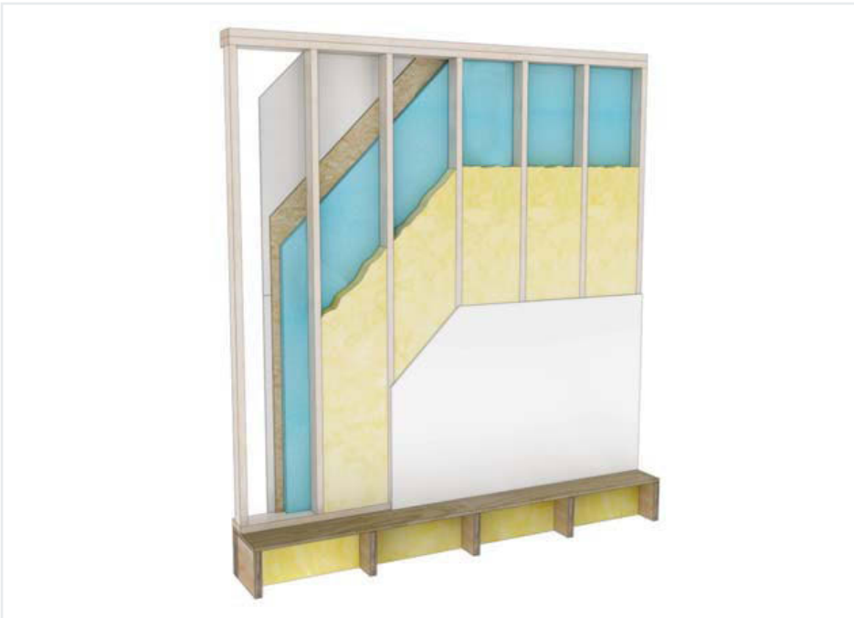
Interior view of the wall system shows the rigid foam (in blue) is interior to the wood structural panel to simplify installation of windows and siding. Illustration from Home Innovation Research Labs
