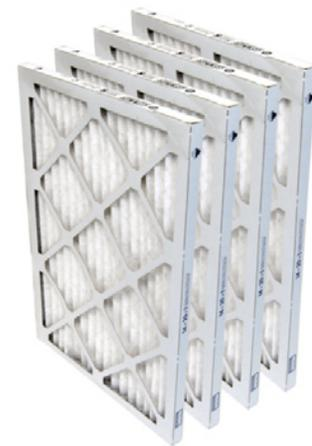
Building America recommends a MERV 8 or higher filter on the HVAC return. MERV (Minimum Efficiency Reporting Value) is a measure of an air filter's efficiency at removing particles. **[This exceeds the ASHRAE 62.2-2010 6.7 recommended MERV 6 or better.]**
