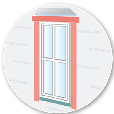
**STEP 8** Install jamb flashing first; install a drip cap (if applicable); install head flashing.
