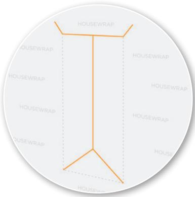
**STEP 4** Install housewrap. Cut modified "I" over window.
