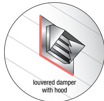
Dryer vent exhausts must have a closeable gravity or automatic damper. A single hinged door with a 2½-inch effective opening is not as effective as a louvered damper.
