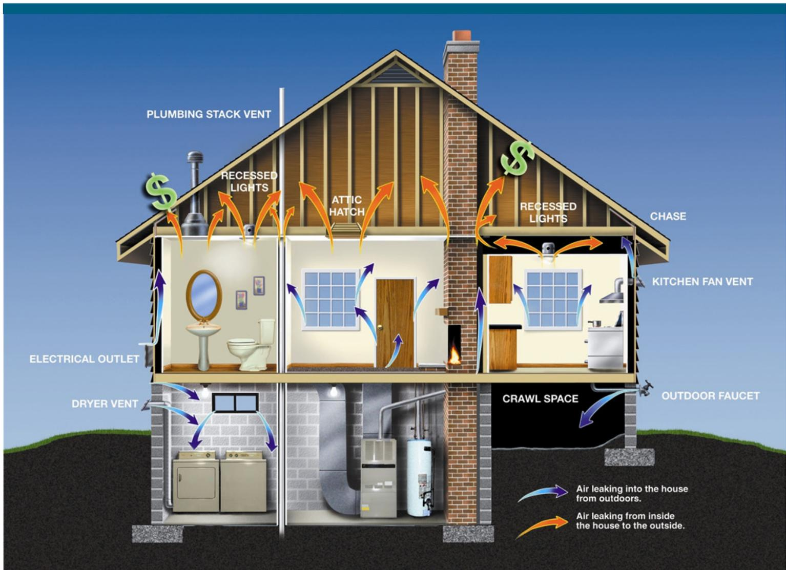
Unintentional air leaks can allow leakage of significant amounts of air into and out of a home in an uncontrolled manner through unsealed seams and unplugged holes in the walls, ceiling, and floors. (Figure source: EPA)
