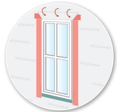
**STEP 9** Fold down head housewrap; apply corner patches at head; air seal window around the entire perimeter on the interior with sealant or non-expanding foam.
