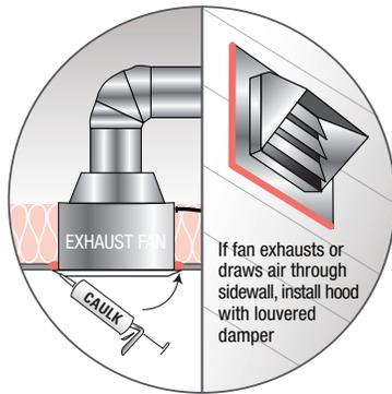
Provide bathroom and kitchen exhaust fans. Duct them to the outside and caulk ducts at the dry wall for an air-tight seal. Use low-sonic fans for quiet operation.
