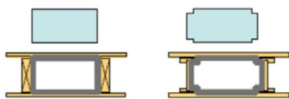
Wood or rigid foam filler blocking is cut to fit the gaps between floor joists and caulked or foamed in place to form an air break between conditioned and unconditioned spaces.
