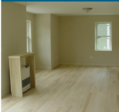
This high-efficiency, sealed-combustion gas space heater heats the entire home at low installation and operating cost.
