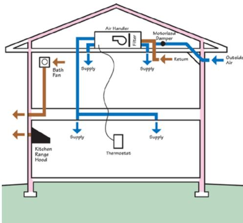
Balanced ventilation system using a fresh air intake integrated with HVAC air handler for supply air and exhaust fans.
