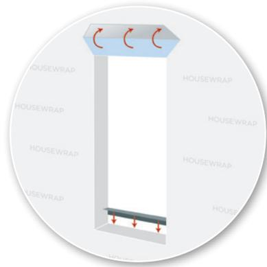
**STEP 5** Fold in housewrap at jambs and sill. Fold back temporarily at jamb. Install backdam on sill.
