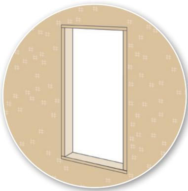
**STEP 1** Rough in window openings, oversizing by 1 ½ inches in both dimensions.
