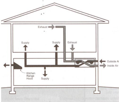
Balanced ventilation system with heat recovery via an air-to-air heat exchanger. (Source: Lstiburek 2004)
