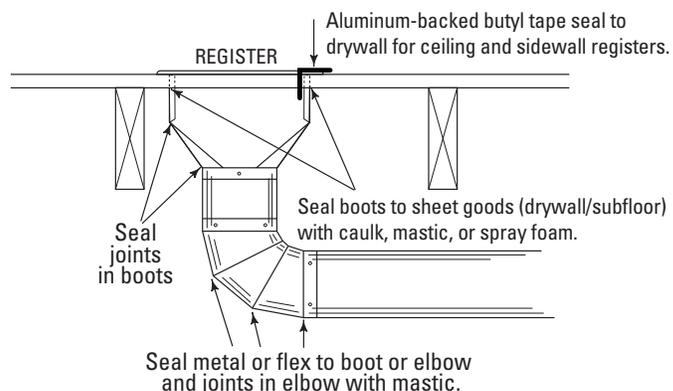
Mastic is a gooey adhesive that is applied wet. It fills gaps and dries to a soft solid. Mastics may or may not contain reinforcing fibers, and they may be used with reinforcing mesh tape.
