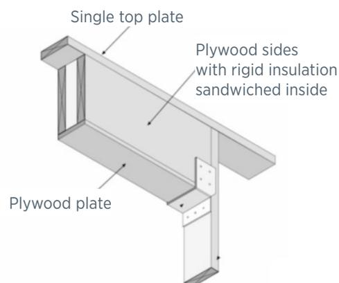
Closed, insulated headers are one advanced framing technique. (Figure source: CARB)
