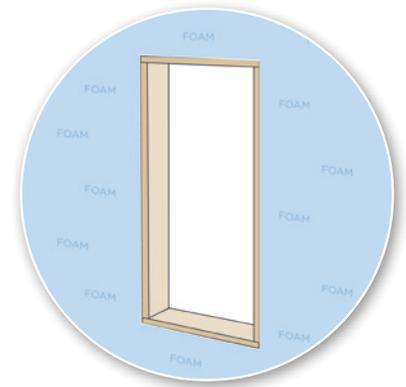
**STEP 3** Install the exterior foam. The outer face of the foam should be flush with the outer edge of the plywood frame.
