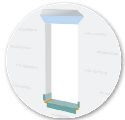
**STEP 6** Install adhesive-backed sill flashing and corner flashing patches at sill. Apply sealant at jambs, head, and sill.
