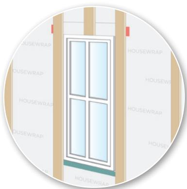
**STEP 10** Install vertical wood strapping on top of the foam and housewrap to use when attaching siding.
