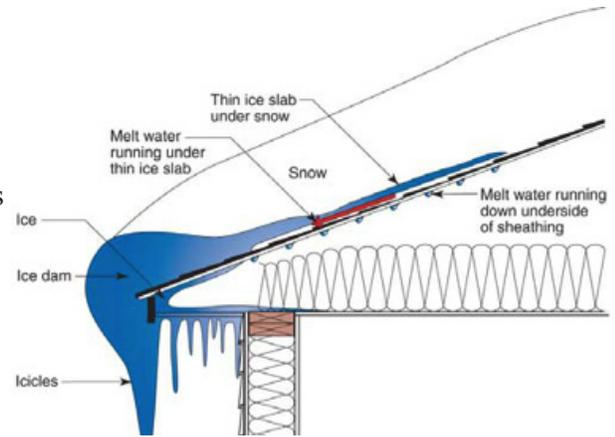
Ice dams can form when the roof deck temperature is above freezing and the air is below freezing. Snow melts, runs down to the edge of the roof and refreezes forming a dam that traps more water and ice. Air leaks in ceilings and insufficient attic insulation allow heat to rise into attic warming roof deck and encouraging ice dam formation.
