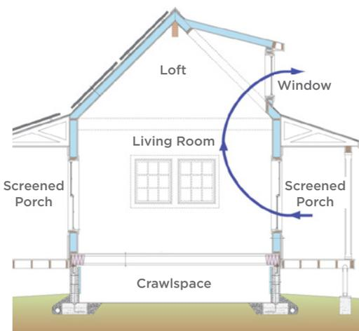
Building America's research team lead Building Science Corporation used convection to help cool this structural insulated panel (SIP) cottage in Georgia. Cool air from the screened porches is drawn into the building's interior where it heats up and is pulled up and out the second-story windows, drawing more air in through the shaded first-story windows.
