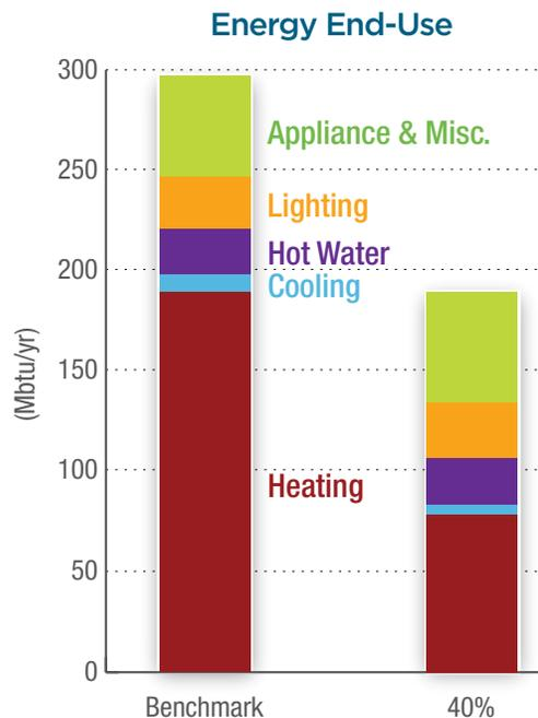
A Comparison of Energy Usage by End Use for a Home Built to Perform with 40% Energy Savings Compared to the Building America Benchmark (a home built to MEC 1993) in the Cold Climate. Example based on a 2-story, 1,354 ft<sup>2</sup> house in Pasco, WA. Analysis by BIRA.
