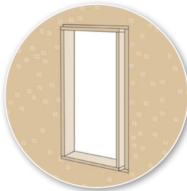
**STEP 2** Line rough opening with a frame made of plywood strips ¾" thick by wall dimension + width of foam (the plywood should be flush on the interior surface and extend to the anticipated outside face of the foam).
