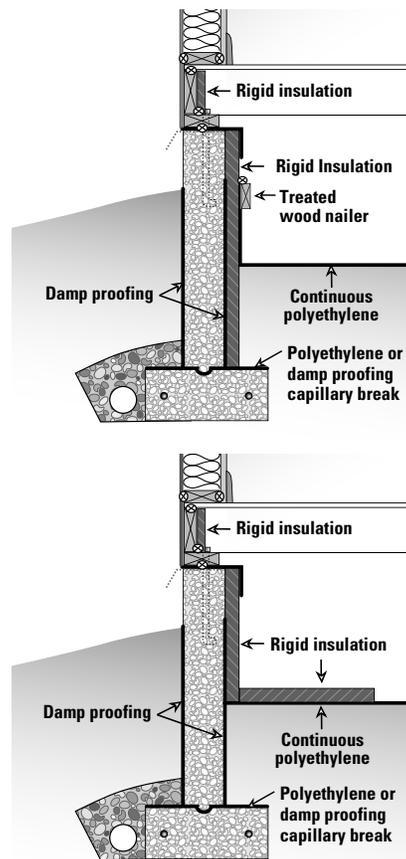
If depth does not extend two feet below grade, place remaining insulation horizontally along the ground.
