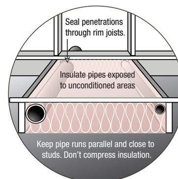
Keep pipes out of exterior walls and seal penetrations through floor.
