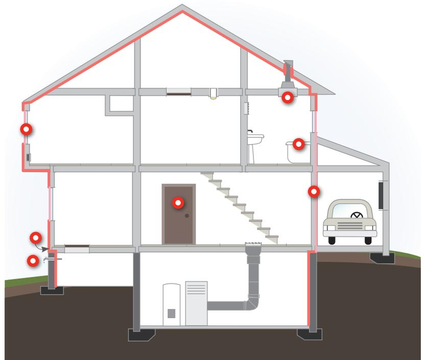
A comprehensive air-sealing strategy begins with indicating on the house plans the location of the conditioned space by outlining the building envelope. The plans should show the location of complex details like chases, stairwells, dropped ceilings, fireplace penetrations, balconies, and knee walls, so that they can easily be identified as being inside or outside the conditioned space. The plans also should show where insulation and draft stopping should be installed.
