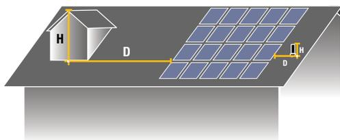
For houses with solar photovoltaic roof panels, any potential shading structure should be twice as far away from the photovoltaic array as it is tall ( $D = 2 * H$ )
