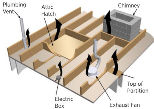
**Figure 5.2. Ceiling holes.** Homes are typically constructed with lots of holes in the ceiling for lights, pipes, vents, ducts, and chimneys. If the builder fails to air seal around these, air escaping through the gaps can carry moisture, possibly leading to mold and wood rot. These gaps must be air sealed before insulation is added to the attic (Figure Source: PNNL).
