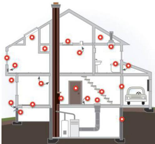
**Air leaks.** There are numerous spots where air can leak into or out of a house, wasting energy and risking problems with moisture and air quality.
