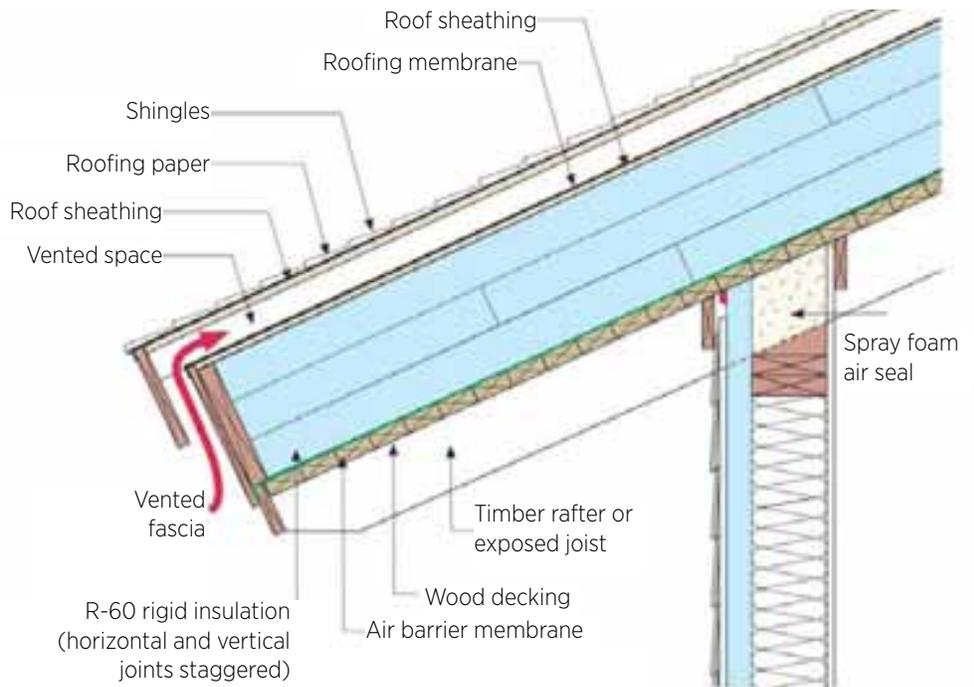
In regions with snow loads greater than 50 lb/ft<sup>2</sup>, the snow can provide enough thermal resistance to allow the roof cladding to be above freezing even when the air temperature is below freezing (one foot of snow = R-10 to R-15). To prevent ice damming with an unvented attic in these conditions, construct a “vented over-roof” over the top of the “unvented compact roof” (Source: Lstiburek 2011).
