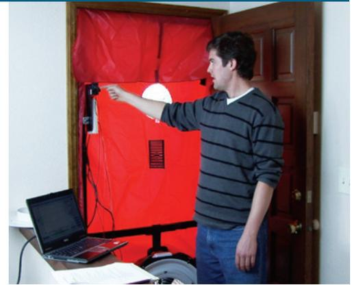
As part of the home performance energy checkup, your certified contractor will use a blower door test to measure whole-house air leakage and determine places where insulation and air sealing are inadequate (Photo Source: PNNL).
