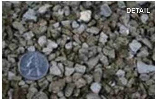
**Vermiculite insulation.** If you have vermiculite insulation in your attic or walls, you should assume that it contains asbestos and be careful to avoid exposure. Vermiculite was commonly used before 1990 (Photo Source: EPA).
