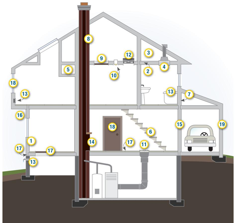
**Figure 5.1. Where to air seal.** Building America research has identified 19 key areas where air sealing can improve a home's energy efficiency, comfort, and durability. A certified home performance contractor can perform a home energy checkup to identify areas in your home that need air sealing (Figure Source: PNNL).
