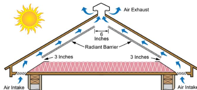
To prevent moisture problems when installing a radiant barrier, leave adequate gaps for air flow above, below, and behind the barrier material.
