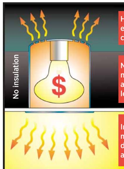
Holes in the top of the recessed can encourage the stack effect, pulling conditioned air up into the attic.
