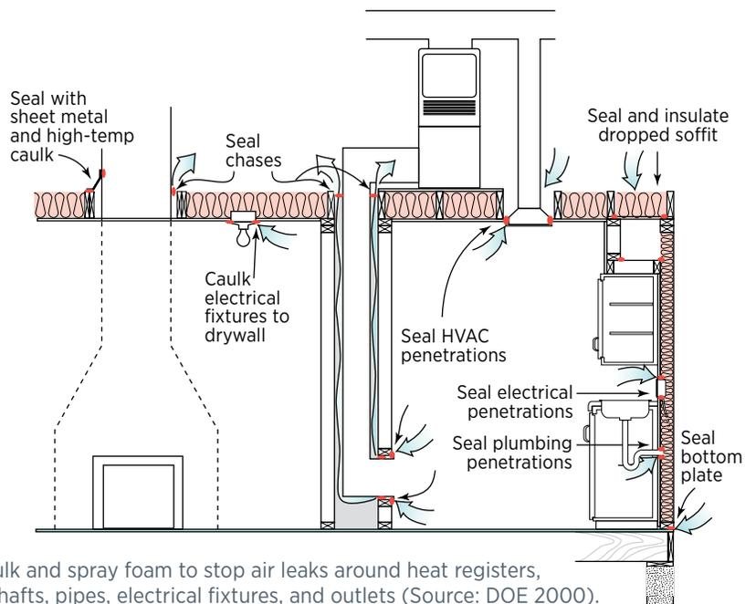
Use caulk and spray foam to stop air leaks around heat registers, ducts shafts, pipes, electrical fixtures, and outlets (Source: DOE 2000).
