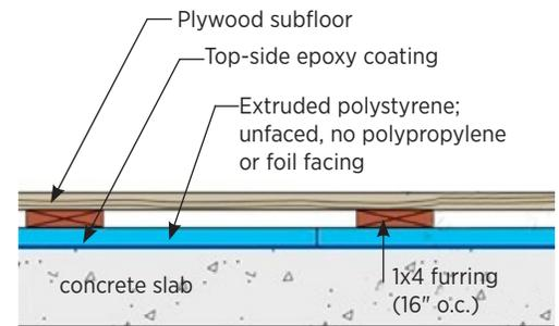
**Figure 5.18. Vapor pressure equalization.**
