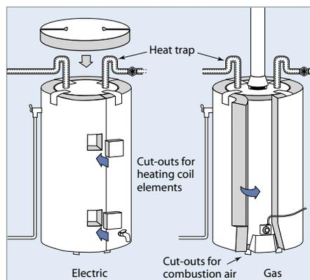
Electric and gas water heaters require different approaches to insulation. Gas and oil-fired water heaters are more difficult to insulate than electric water heaters. Their installation may be best handled by a qualified plumbing or heating contractor.
