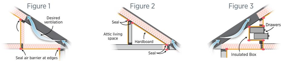
Figure 1. Insulate and air seal the kneewall (Source: DOE 2000).
