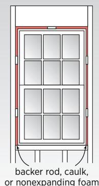
Figure 18.1. Use backer rod, caulk, or nonexpanding foam approved for windows and doors to fill the rough-in gap around doors and windows (DOE 2000).
