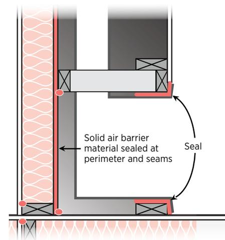
Figure 14.1. Air seal the enclosure surround and flue.
