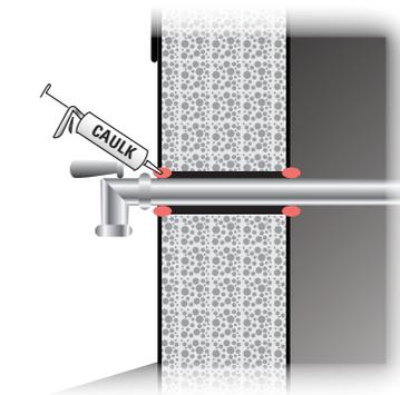
Figure 13.1. Caulk all plumbing penetrations through exterior walls.
