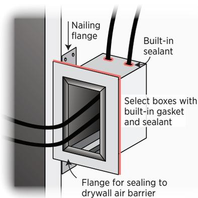
Figure 13.3. Seal all electric outlets and switches with foam sealant, or select boxes with built-in sealant or gaskets. Install foam gaskets between electrical outlets or switches and their coverplates, and insert plastic “child-safety” plugs into the outlets to further block airflow.
