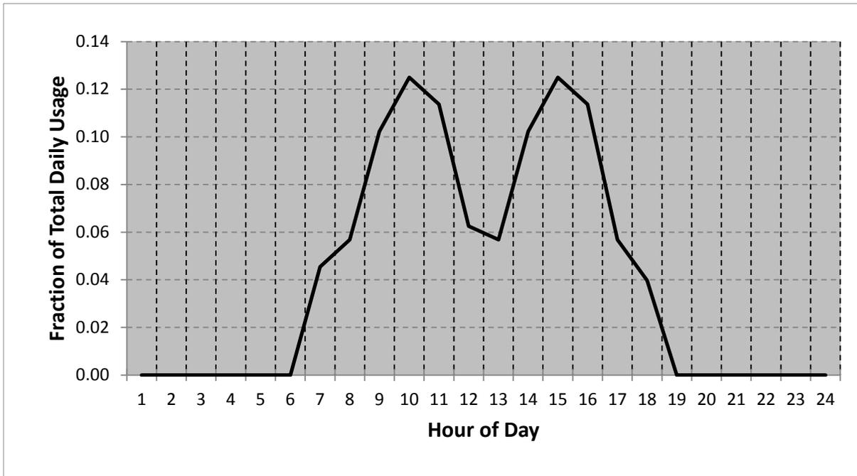
Figure 12. Central restroom sink hot water use profile
