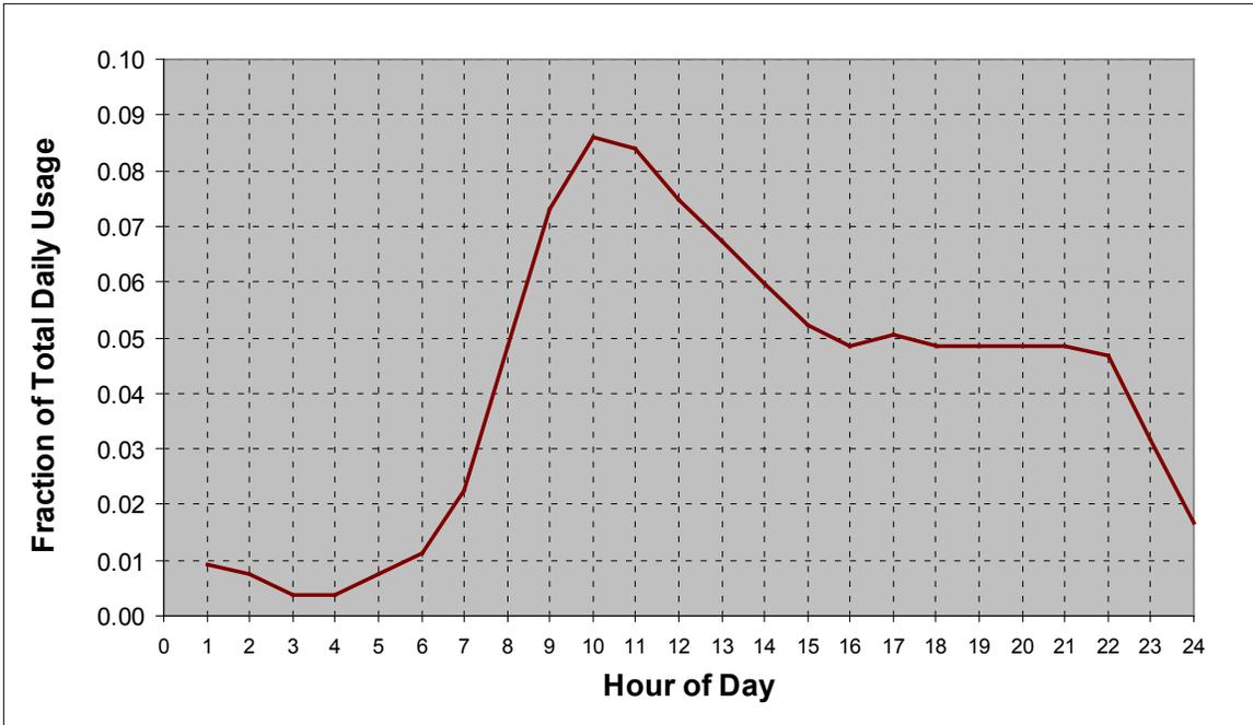
**Figure 17. Clothes washer normalized machine energy use profile**
