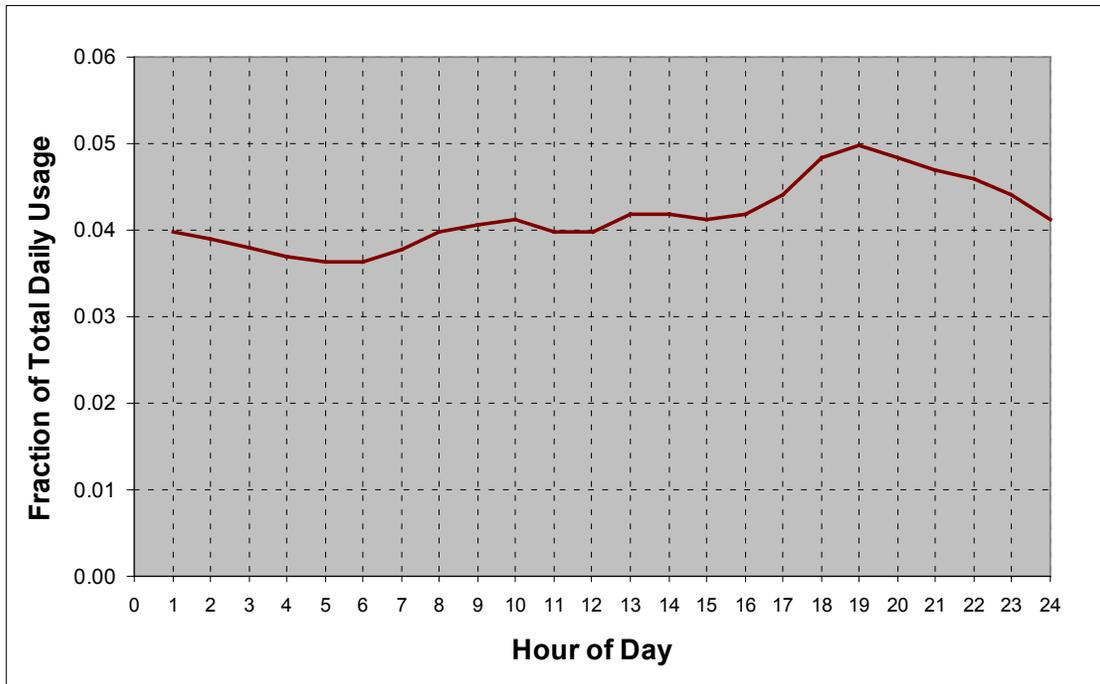
**Figure 16. Refrigerator normalized energy use profile**
