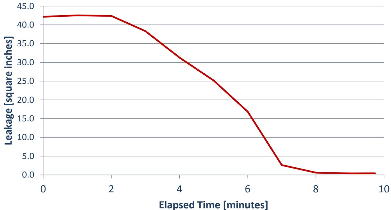
**First Test:** Using 100 ccm sealant, and no pressure control
