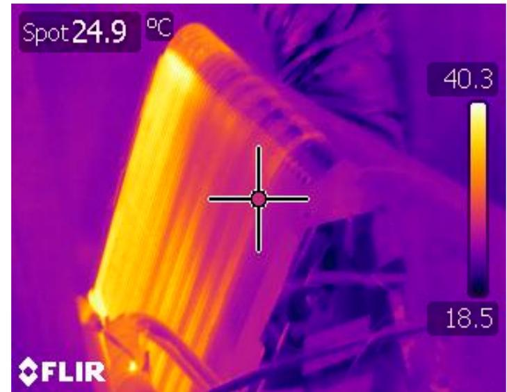
*House B refrigerant coil in heating mode showing non-uniform temperatures*
