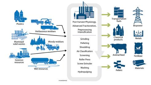
Feedstock Supply and Logistics R&D is developing technologies with a vision to expand preprocessing operations to provide multiple high- and low-value feedstock streams. Image courtesy of Idaho National Laboratory.
