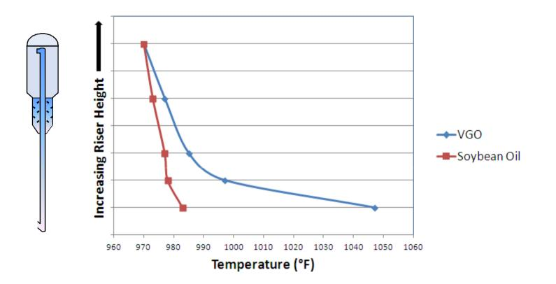
Same preheat, catalyst temperature and riser outlet temperature.
