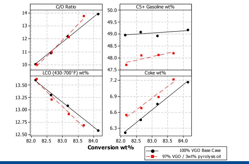
Adding pyrolysis oil results in more coke, less gasoline and less LCO.
