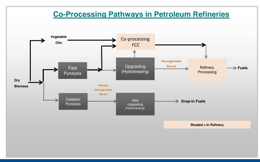
There are multiple pathways for co-processing biomass in refineries.
