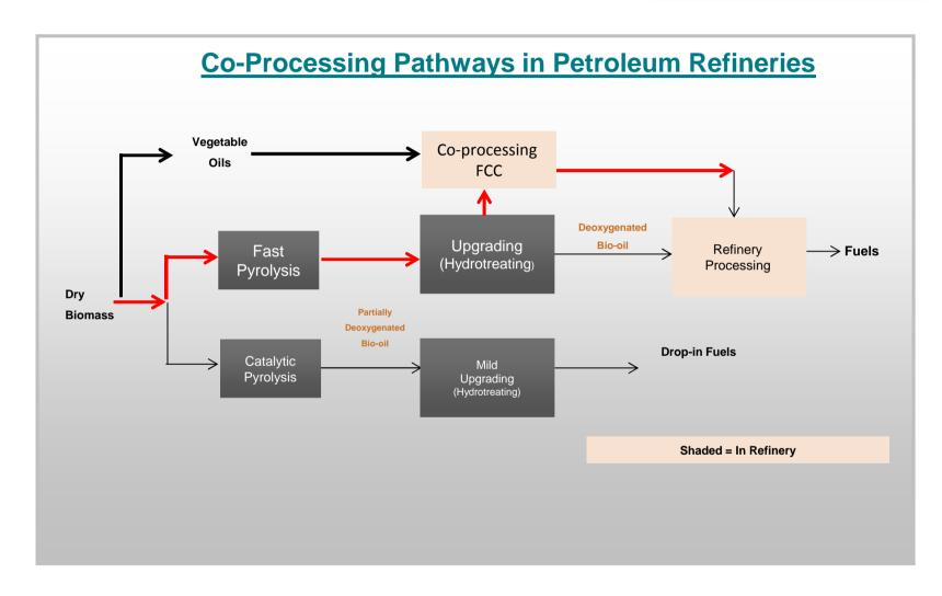
Pyrolysis Oils will require upgrading (hydrotreating) prior to processing in FCC
