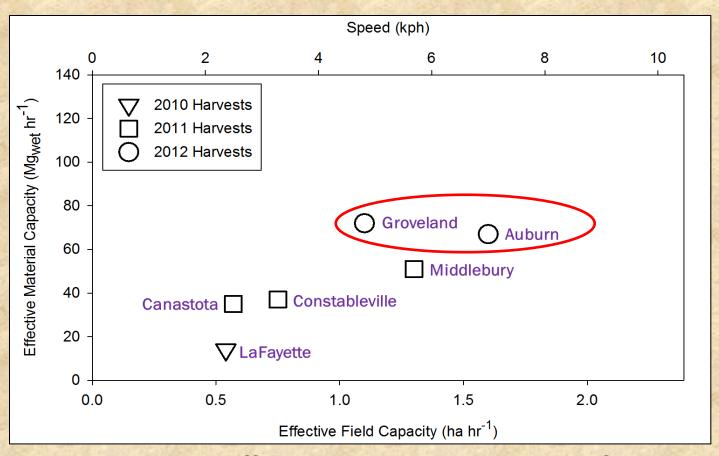
Improvements in effective material capacity for several willow harvests from below 20 Mg<sub>wet</sub> hr<sup>-1</sup> to about 70 Mg<sub>wet</sub> hr<sup>-1</sup> as observed over the three-year project.
