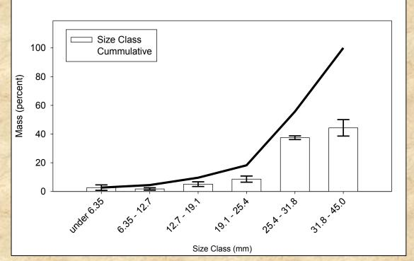
Particle size distribution of willow biomass samples collected during harvesting trials in 2012/13. Error bars indicate one standard deviation.
