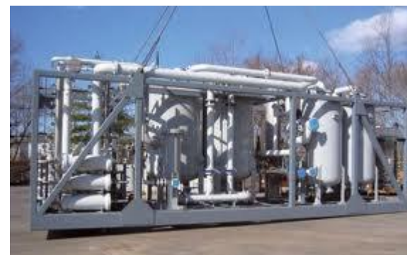
Membrane Biogas Cleaning Courtesy of Air Liquide
