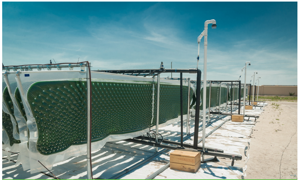
Algenol Biotech, LLC cultivates spirulina in photobioreactors at a facility in southwest Florida. Photo from Algenol Biotech LLC.
