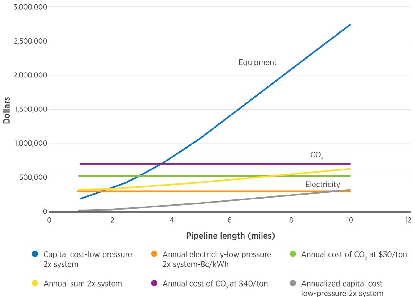
**Figure D-4** | Equipment and electricity costs for coal flue gas transport system, including two parallel sets of pipelines and blowers. The system supports a 1,000-acre open pond and is designed to minimize cost.
