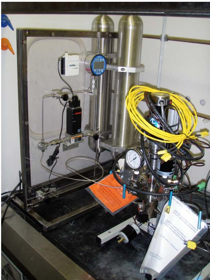
Reservoirs allow H<sub>2</sub> uptake measurement at constant pressure,
