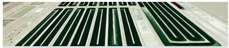
Algae are often grown in outdoor raceway ponds to ensure adequate exposure to sunlight. Research suggests biofuels from microalgae alone could displace 17% of today's transportation fuel imports. *Photo: Pacific Northwest National Laboratory (PNNL)*
