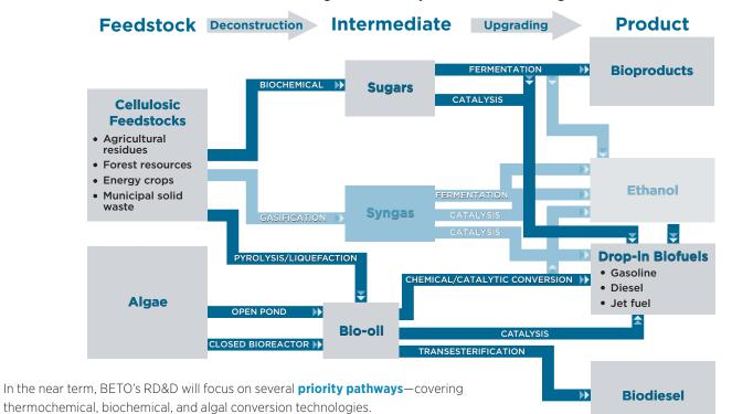
The Bioenergy Technologies Office is concentrating high-value, high-risk RD&D on the key conversion pathways for deconstructing biomass into sugars and bio-oils and then upgrading those intermediates into advanced hydrocarbon fuels. *Chart by Energetics Incorporated*
