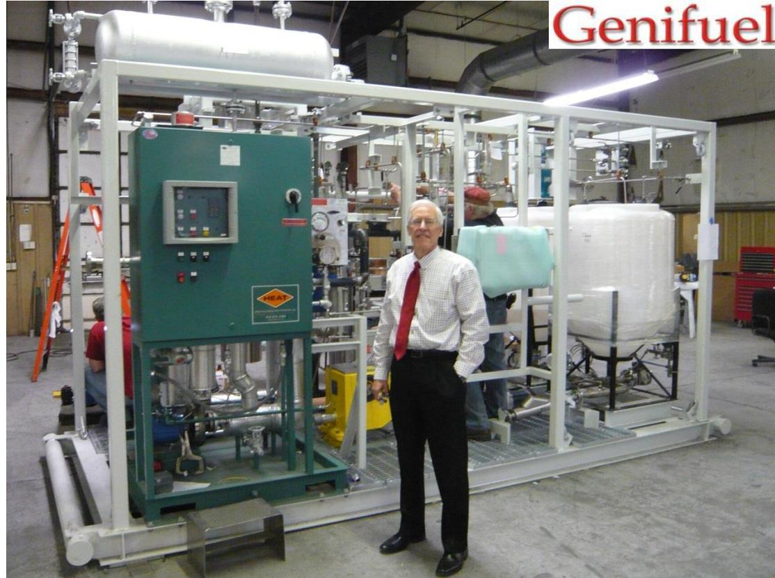
Jim Oyler with the 1000 L/day (of 20 wt% BDAF) Hydrothermal Processing Pilot System continuous HTL/CHG system for algal feedstock NAABB-Reliance-PNNL-Genifuel
