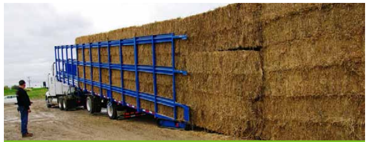
FDC Enterprises' self-loading/unloading trailer, developed with BETO funding in partnership with Kelderman Manufacturing, can pick up a stack of 36 corn stover bales in five minutes.
