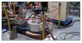
The BioChemCat process employs a unique combination of process steps, which include: pretreatment technology (wet oxidation); fermentation using a mixed anaerobic consortium to produce platform molecules; separation of platform molecules; and catalysis reactions for upgrading the platform molecules into hydrocarbons. The key outcome of the project is the maturation of a
