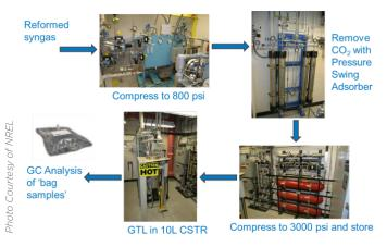
This project demonstrated the integrated production of cost-competitive ethanol from mixed alcohols produced from biomass-derived syngas at pilot scale. The objectives of the project were to integrate the unit operations; evaluate the performance of all unit operations using
