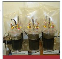
The purpose of this research was to increase renewable energy production via anaerobic co-digestion of municipal wastewater biosolids with various biomass residuals. In co-digestion, a mixture
