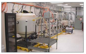
The University of Nevada, Las Vegas and an industrial partner, Ceramatec, are developing a tubular Sodium Super Ionic Conductors (NaSICON) membrane-based process that produces high-purity sodium methoxide from low-cost aqueous sodium hydroxide. An electric
