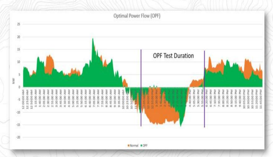
Power at Transformer set to 0 Watts throughput. System set to aggregated optimization.
