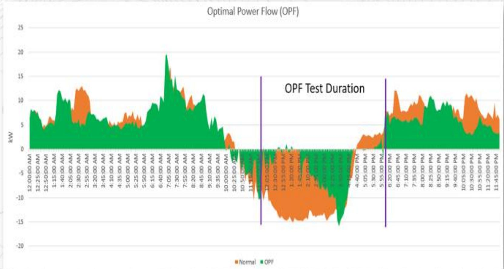
Power at Transformer set to 0 Watts throughput. System set to aggregated optimization.
