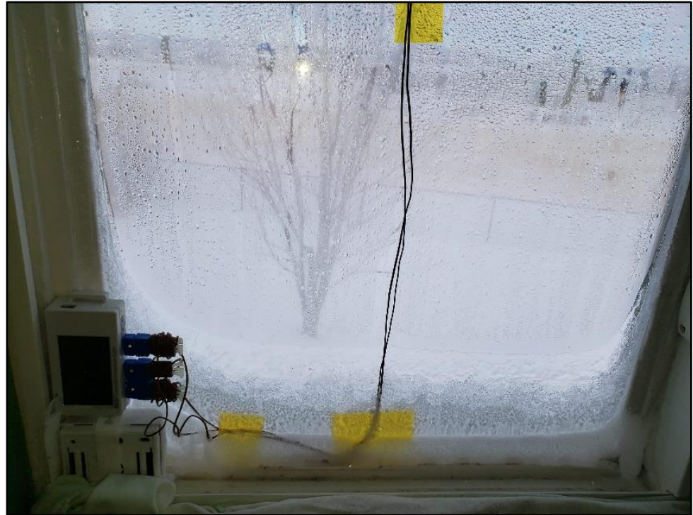
Condensation and ice buildup on interior surface of Helena, MT home field site (double-pane code window).
