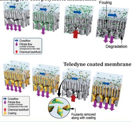
A protective coating (yellow) on the polymer membrane provides chemical and fouling resistance. Removing the foulants and/or coating during chemical backflush and subsequent in-place regeneration increases longevity. *Graphic image credit Teledyne.*
