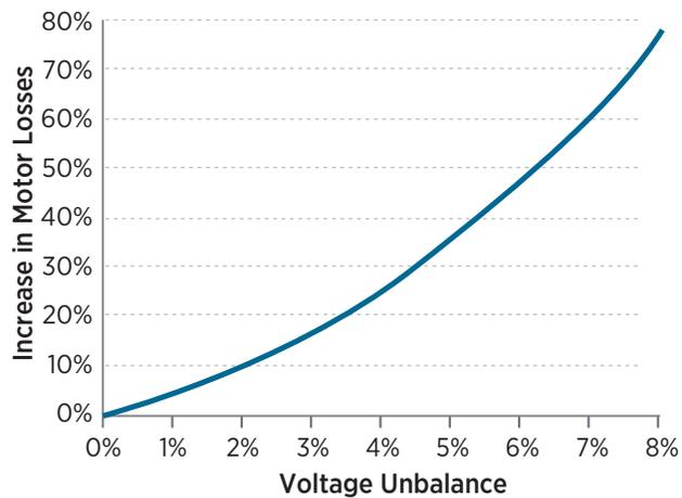
Figure 5-3. Effects of voltage unbalance on motor losses
