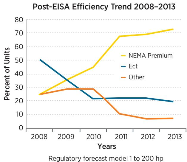
Figure 1-1. Motor sales trends by efficiency class<sup>1</sup>
