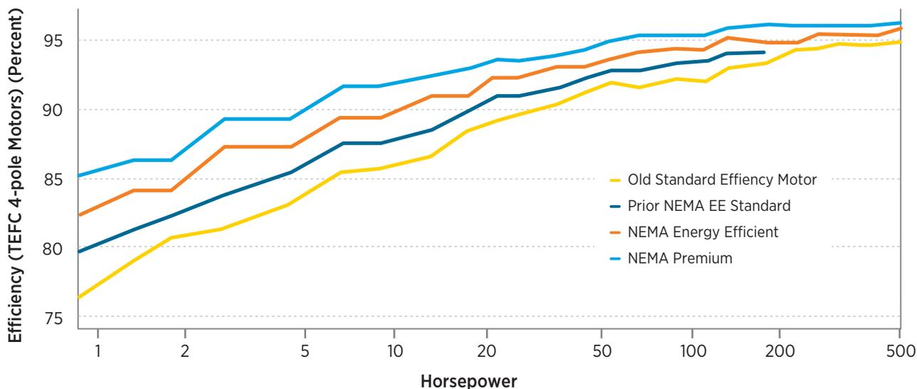
Figure 2-1. Standard, energy-efficient and premium efficiency motor performance
