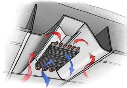
Figure 1: Passive Chilled Beam Design
