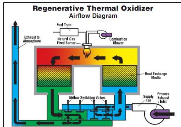
Figure 1: Airflow of an RTO
