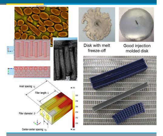
The project explored the design and fabrication of composite heat exchangers through material characterization and modeling. Image courtesy of United Technologies Research Center.
