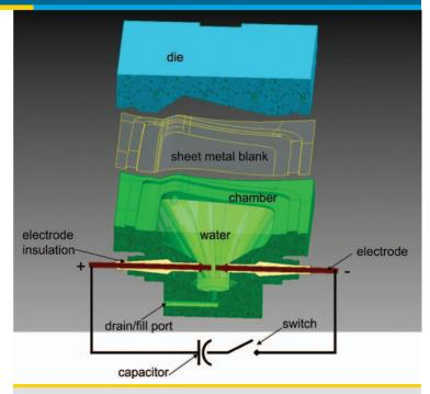
Schematic of the electrohydraulic forming process. The electrohydraulic effect is created via a shock wave generated by the discharge of high-voltage capacitors through a pair of electrodes in a liquid-filled chamber.
