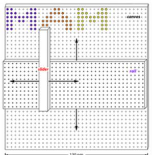
Stepper motors move 3.5 nm per transition in response to externally triggered pulses of short DNA strands.
