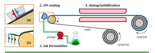
Process overview of the Simultaneous Multilayer Roll-to-Roll (SM-R2R) coating from highly particulate loaded aqueous inks (HIPLAIs). Two types of SM coating dies are depicted in insets: (a) 2-layer slot die coating and (b) 3-layer slide coating. *Photo credit Saint-Gobain Ceramics and Plastics, Inc.*
