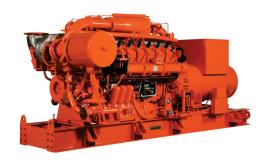
Fig 3. Waukesha's APG1000 Enginator is a turbocharged and intercooled, sixteen cylinder, lean combustion gaseous fueled engine system. *Photo courtesy of GE Dresser Waukesha*.
