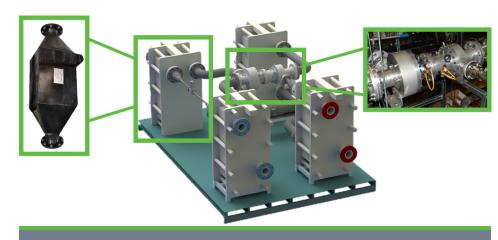
The turbo-compression cooling system being developed utilizes high efficiency turbomachinery and a new type of liquid-coupled aluminum heat exchanger that provides a large amount of surface area at a low cost. *Photo credit Modine Manufacturing Company.*
