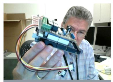
Project partners developed intelligent system control hardware and software for the residential gas heat pump. Photo courtesy of Oak Ridge National Laboratory
