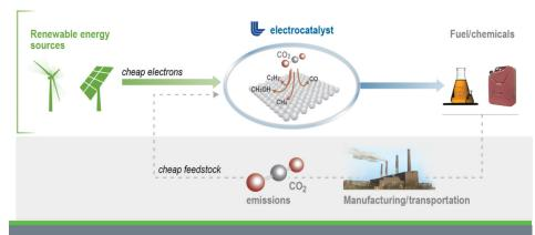
Using electric energy from renewable energy sources, the copper-based electrocatalysts developed through this project would enable one-step conversion of  ${\rm CO}_2$  to methane and other versatile fuels and feedstock chemicals. *Graphic image courtesy of Lawrence Livermore National Laboratory*
