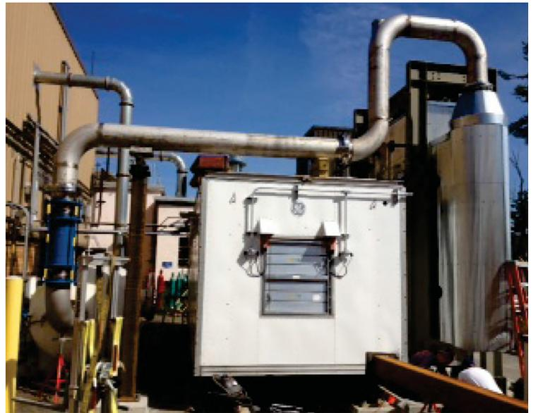
The direct evaporator and supporting equipment installed at the GE test facility. *Photo courtesy of Idaho National Laboratory.*
