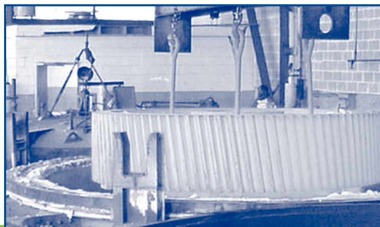
This large-diameter gear was heat-treated at the Metlab facility in Wyndmoor, Pennsylvania.
