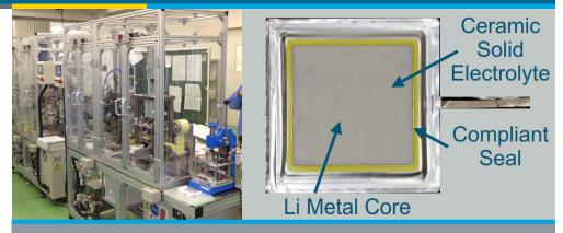
The pilot scale manufacturing line for protected lithium electrodes was designed, built, installed, and optimized during this project (left) in order to manufacture water-stable protected lithium electrodes (right). *Courtesy of PolyPlus.*
