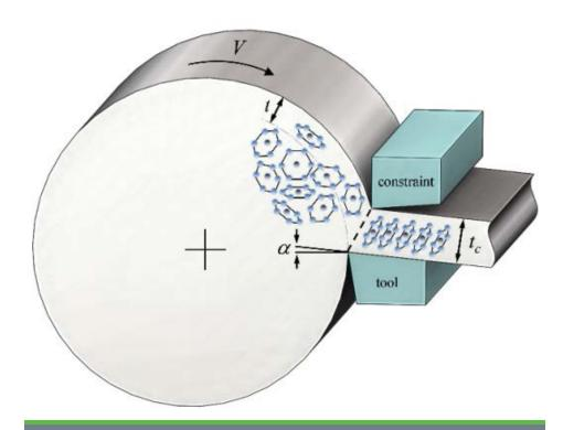
The single-stage cutting-extrusion process to manufacture sheet metal has been developed at Purdue University. It has been used successfully at the laboratory scale to manufacture narrow strips of high silicon content steel. *Graphic courtesy of Purdue University*
