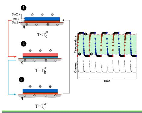
(Left) Thermal oscillators Sw1 and Sw2 act in tandem to periodically vary the temperature of the pyroelectric layer. The current output is proportional to the rate of change of temperature (right), shown here schematically using an exponential form.
