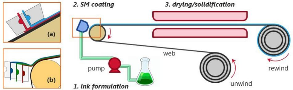
Process overview of the Simultaneous Multilayer Roll-to-Roll (SM-R2R) coating from highly particulate loaded aqueous inks (HIPLAIs). Two types of SM coating dies are depicted in insets: (a) 2-layer slot die coating and (b) 3-layer slide coating.
