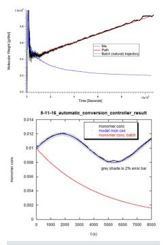
Figure 2. First ever automatic feedback control of molecular weight during polymerization, top, shows linearly increasing target Mw trajectory (red), and the reaction that followed it (black). Automatic control of conversion (black) along a sinusoidal target trajectory (blue) is shown in the bottom graph
