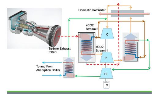
To achieve full-load and partial load efficiency targets, the CHP system will incorporate two cascading bottoming cycles that utilize supercritical carbon dioxide  $(sCO_2)$  as the working fluid. Image courtesy of Siemens Corporation
