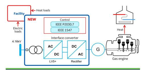
A schematic detailing the key technologies being developed: A converter-interface consisting of a rectifier and grid-ready inverter with an integrated controller.
