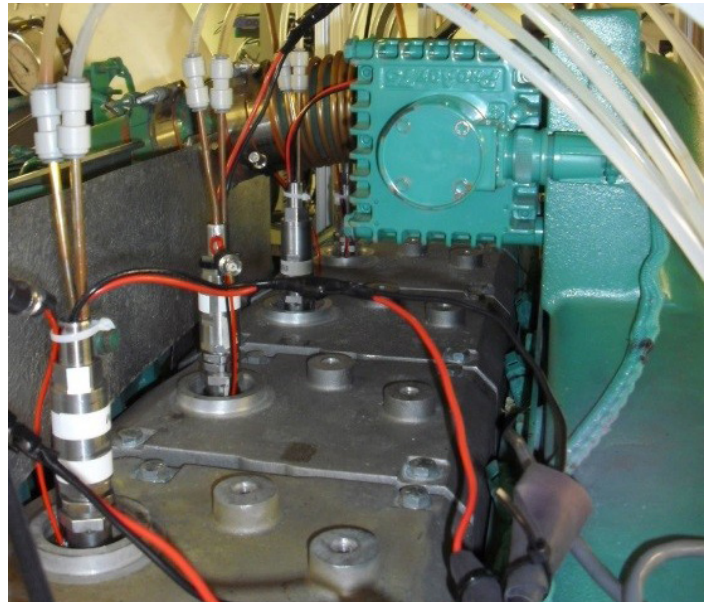
Laser igniters being tested on a 6-cylinder natural gas engine. Laser ignition benefits include higher engine efficiency and the ability to meet stricter emissions regulations. Photo courtesy of Argonne National Laboratory.
