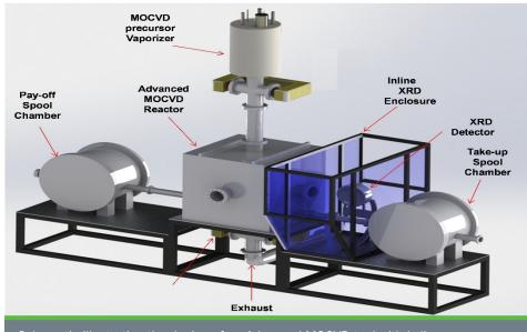
Schematic illustrating the design of an Advanced MOCVD tool with in-line x-ray diffraction (XRD) system for real-time Quality Control at the University of Houston. *Photo credit The University of Houston.*
