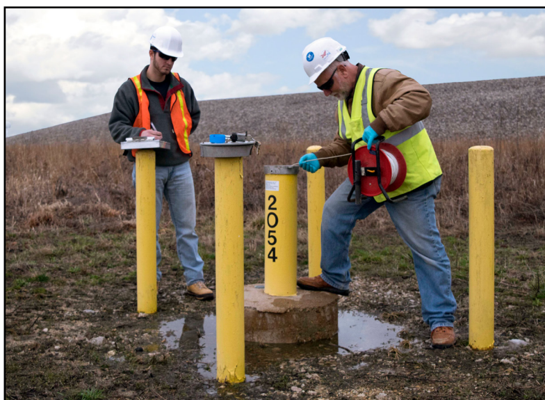
Workers taking a groundwater sample at the Weldon Spring Site.
