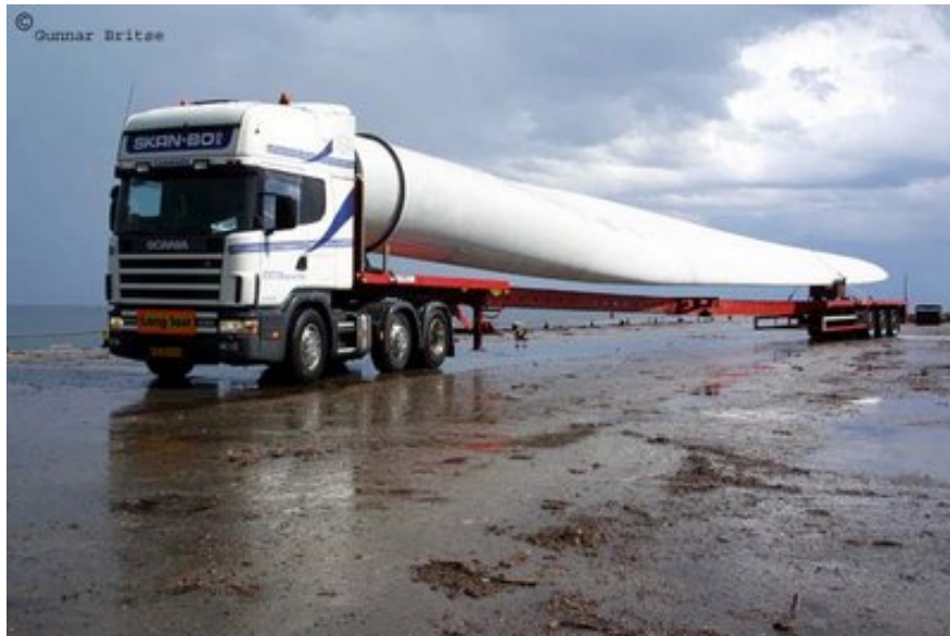
Figure 7 – Truck load with one 2.5 MW turbine blade.
