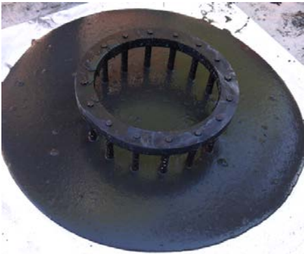
Passing ability test (J-ring)
