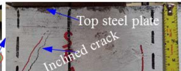
(b) Crack close top steel plate
