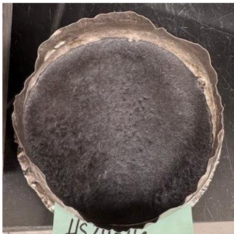
Figure E.16. Glass HS24-16 morphology after CCC.
