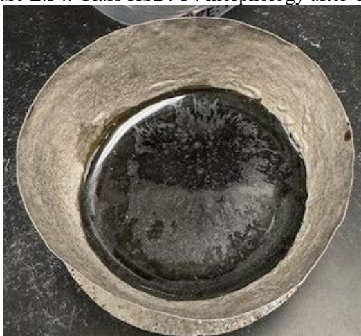
Figure E.35. Glass HS24-35 morphology after CCC.
