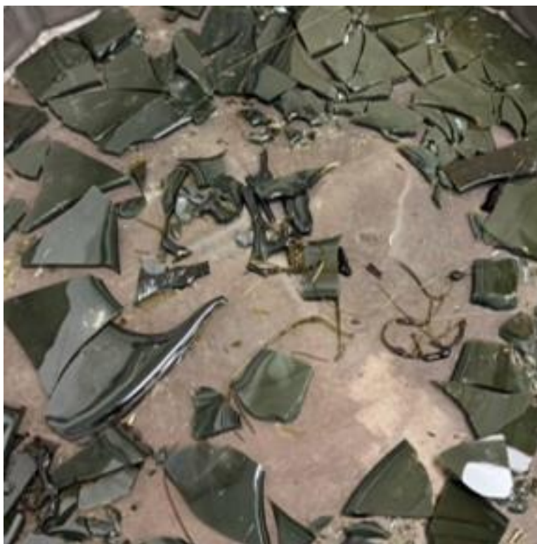
Figure B.29. Photographs of HS24-29 after the second melt using a tilt-pour furnace.
