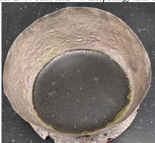
Figure E.50. Glass HS24-50 morphology after CCC.
