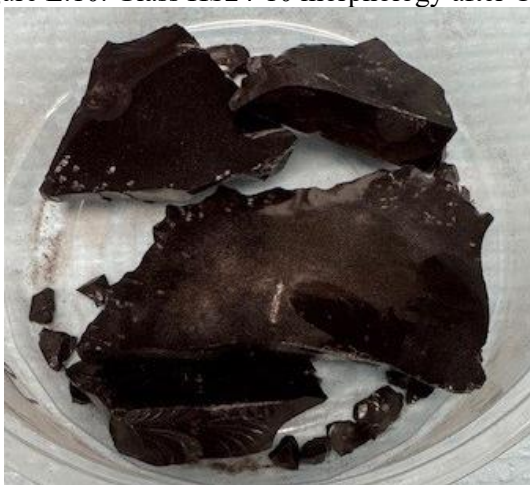
Figure E.11. Glass HS24-11 morphology after CCC.
