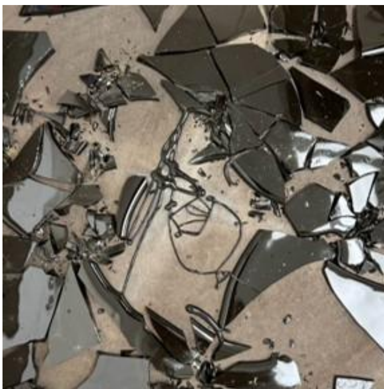
Figure B.3. Photographs of HS24-03 after the first melt using a tilt-pour furnace.
