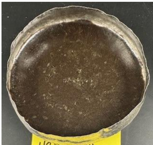
Figure E.28. Glass HS24-28 morphology after CCC.
