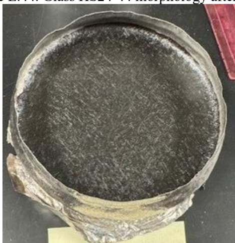
Figure E.45. Glass HS24-45 morphology after CCC.
