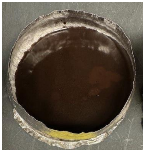
Figure E.22. Glass HS24-22 morphology after CCC.
