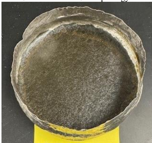
Figure E.30. Glass HS24-30 morphology after CCC.
