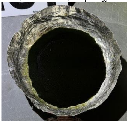
Figure E.14. Glass HS24-14 morphology after CCC.
