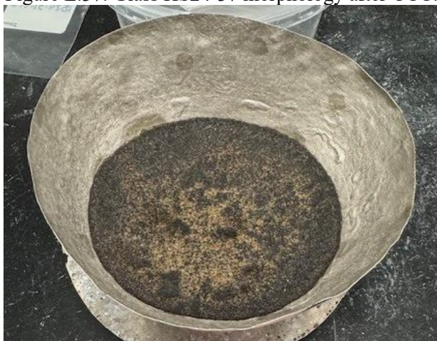
Figure E.38. Glass HS24-38 morphology after CCC.
