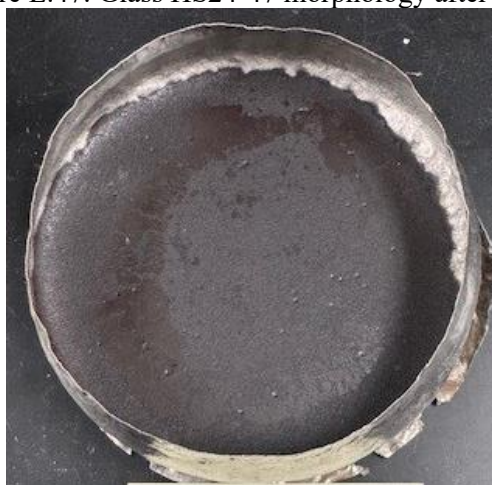
Figure E.48. Glass HS24-48 morphology after CCC.
