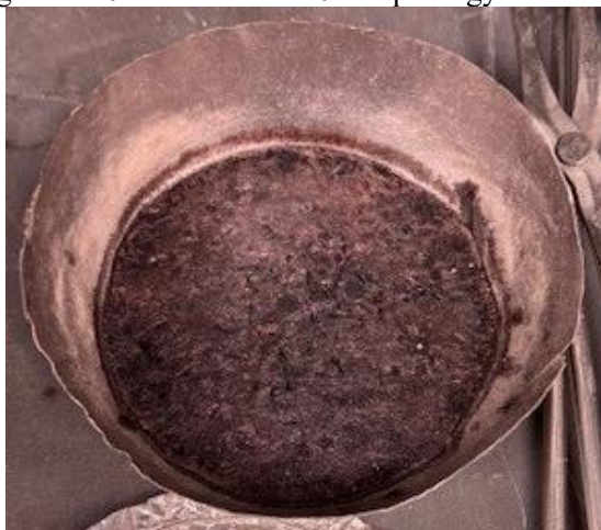
Figure E.21. Glass HS24-21 morphology after CCC.
