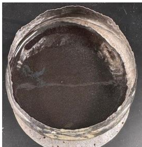
Figure E.46. Glass HS24-46 morphology after CCC.
