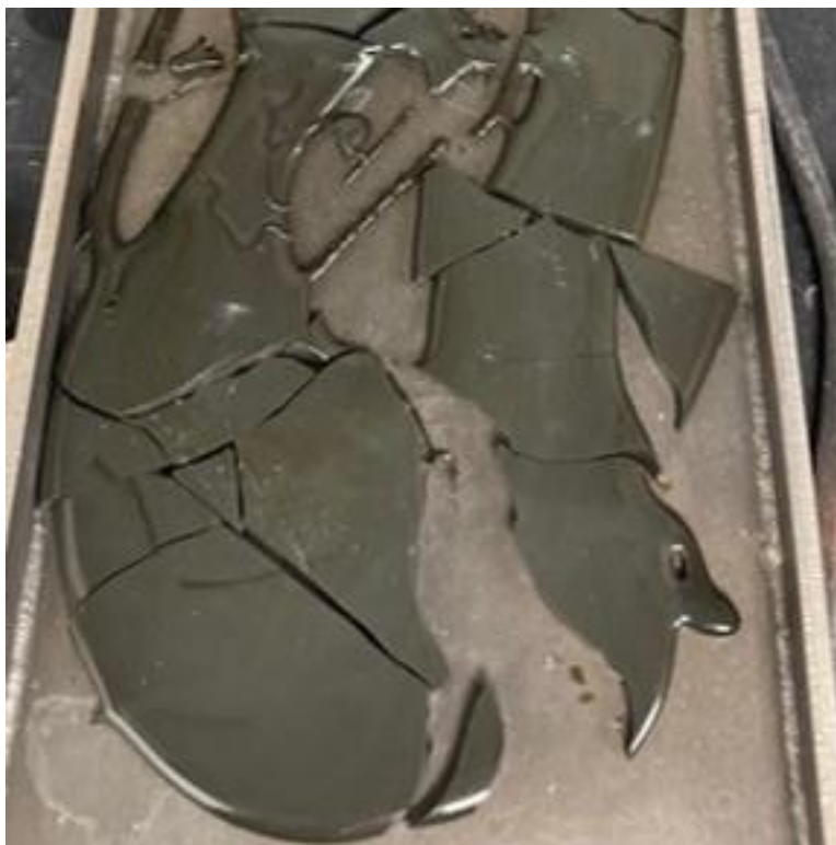
Figure B.28. Photographs of HS24-28 after the third melt using a Deltech furnace.
