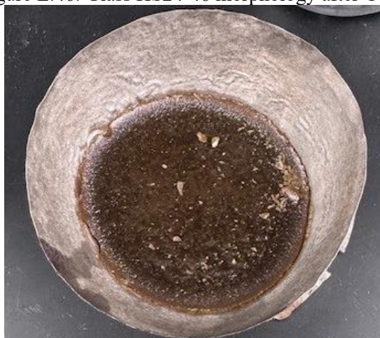
Figure E.47. Glass HS24-47 morphology after CCC.
