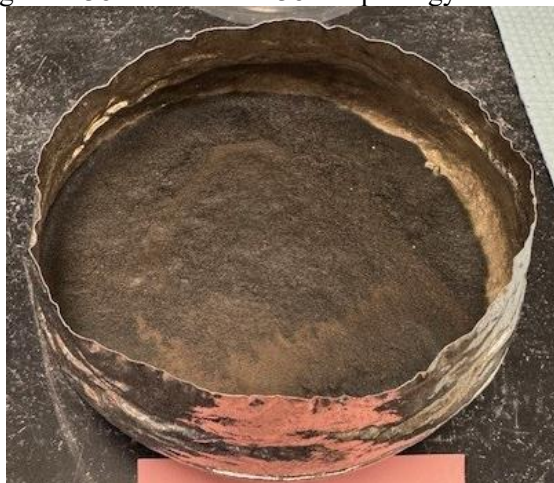
Figure E.39. Glass HS24-39 morphology after CCC.
