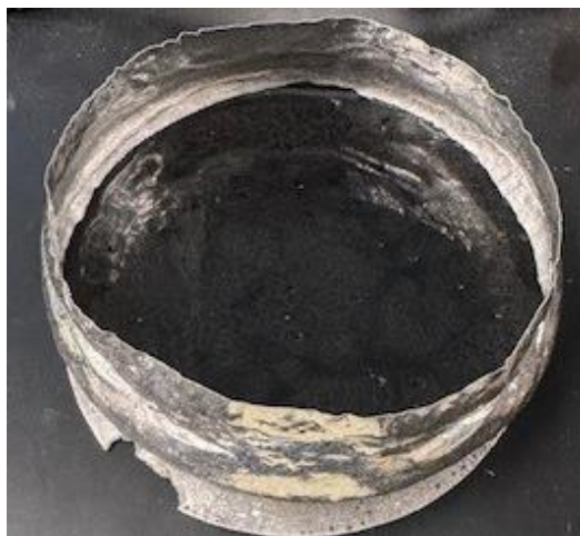
Figure E.43. Glass HS24-43 morphology after CCC.
