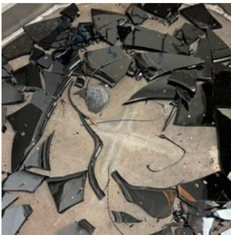
Figure B.21. Photographs of HS24-21 after the second melt using a tilt-pour furnace.
