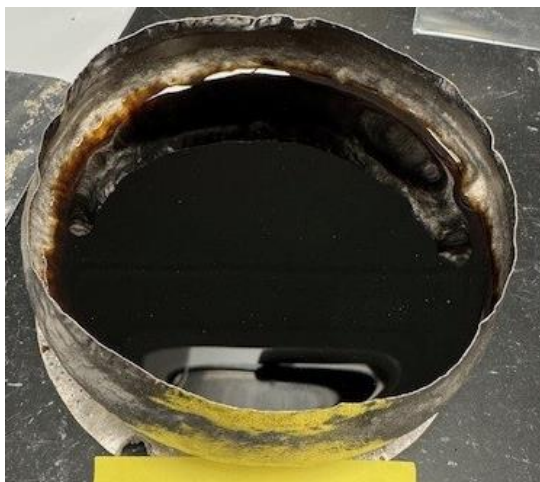
Figure E.37. Glass HS24-37 morphology after CCC.
