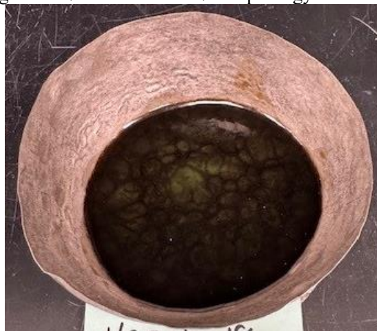
Figure E.18. Glass HS24-18 morphology after CCC.
