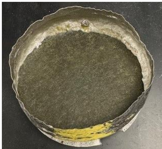
Figure E.34. Glass HS24-34 morphology after CCC.
