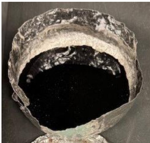
Figure E.19. Glass HS24-19 morphology after CCC.
