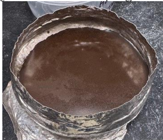
Figure E.42. Glass HS24-42 morphology after CCC.
