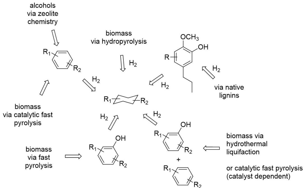
Figure 16. Routes to cyclohexanes that can be synthesized in the jet-fuel range
