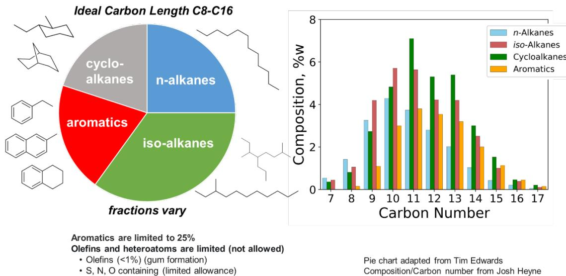
**Figure 5. Composition of an average Jet A (POSF 10325) (Edwards 2017).** *n*-Alkanes, iso-alkanes, cycloalkanes, and aromatics are approximately normally distributed across the carbon number range. A molecule with 11 to 12 carbons is approximately average.
