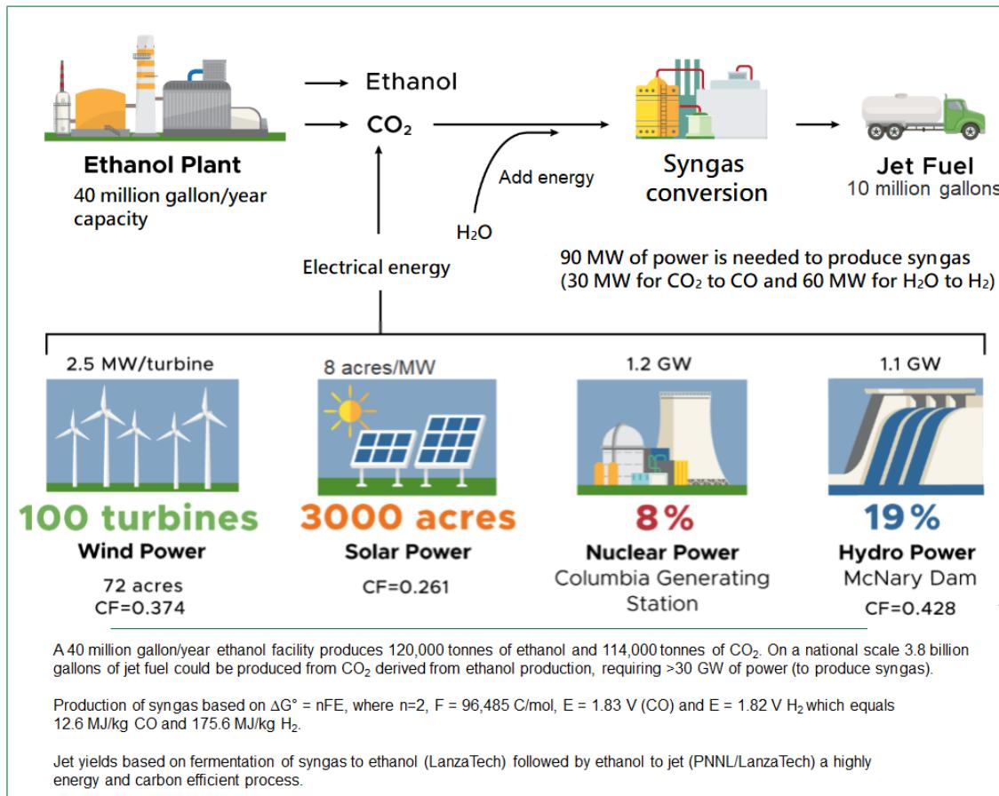
Figure 20. CO<sub>2</sub> from ethanol production conversion to jet fuel via synthesis gas
